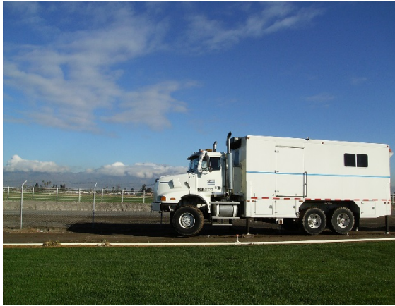
Cone penetrometer testing/pore pressure testing used to map subsurface lithology and locate water-bearing geologic units below the Airport Property .
