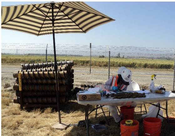
Geologist performing field tests and methodologies to identify soil types, log subsurface lithology, and locate water-bearing strata for groundwater sampling and final well design.
