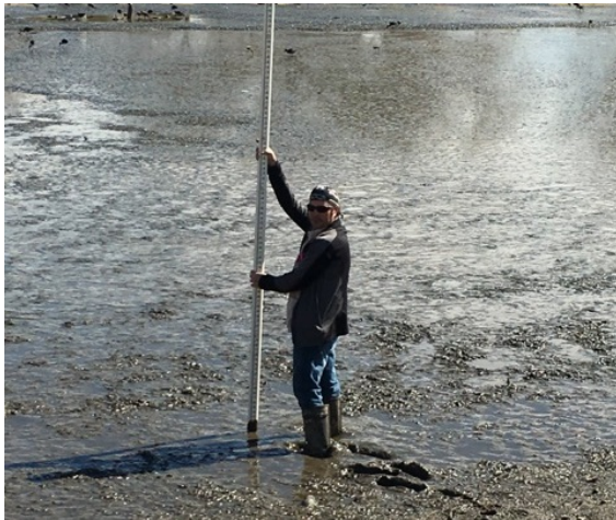
Field technician measuring depth to the lake bottom at El Prado Regional Park south of the Airport .
