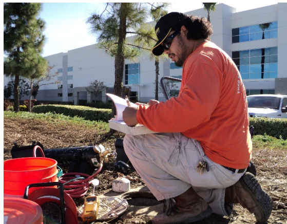
Field technician collecting samples from groundwater wells at off- Site wells southwest of the Airport .
